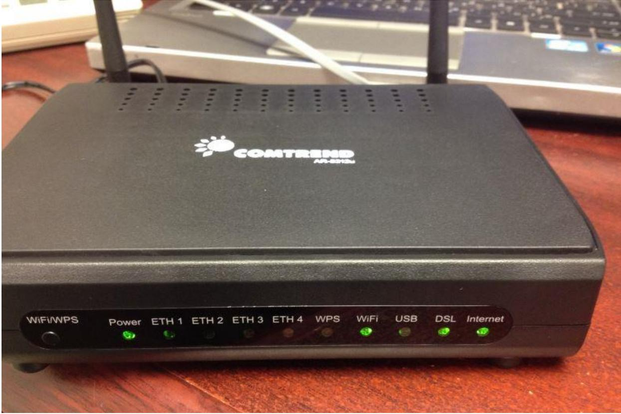
If your Geetel DSL modem is a black Comtrend AR-5312u or AR-5319 wireless modem/router combination, the lights across the front of the modem are as follows:
